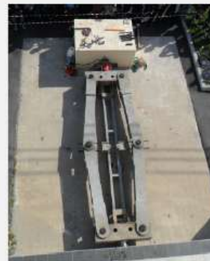
Snap-back testing of a base isolated building - Italy, Augusta, 2013
