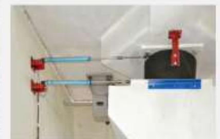
Snap-back testing of a base isolated building - Italy, Augusta, 2013
