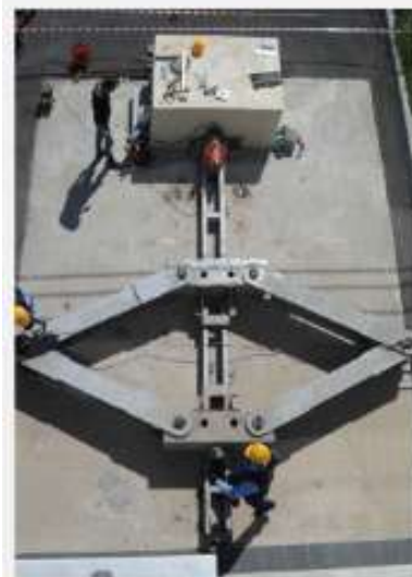
Snap-back testing of a base isolated building - Italy, Augusta, 2013
